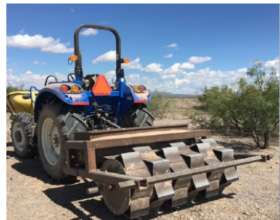
Tractor with imprinter. Source: Lordsburg Playa Watershed Restoration to Reduce the Severity of Dust Storms on I-10.
