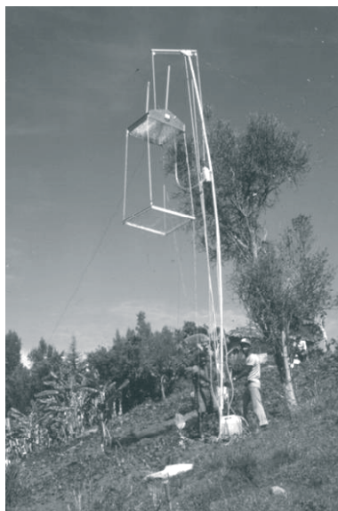
Figure 4. Rain simulator (left) and infiltration envelope. Lower infiltration capacity corresponds to shift of the envelope to the left
