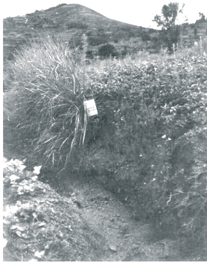
Figure 9. On steep slopes, the pressure by sediments retained by the hays is too high. The hay is pushed forward and finally fails as happened in the foreground.
