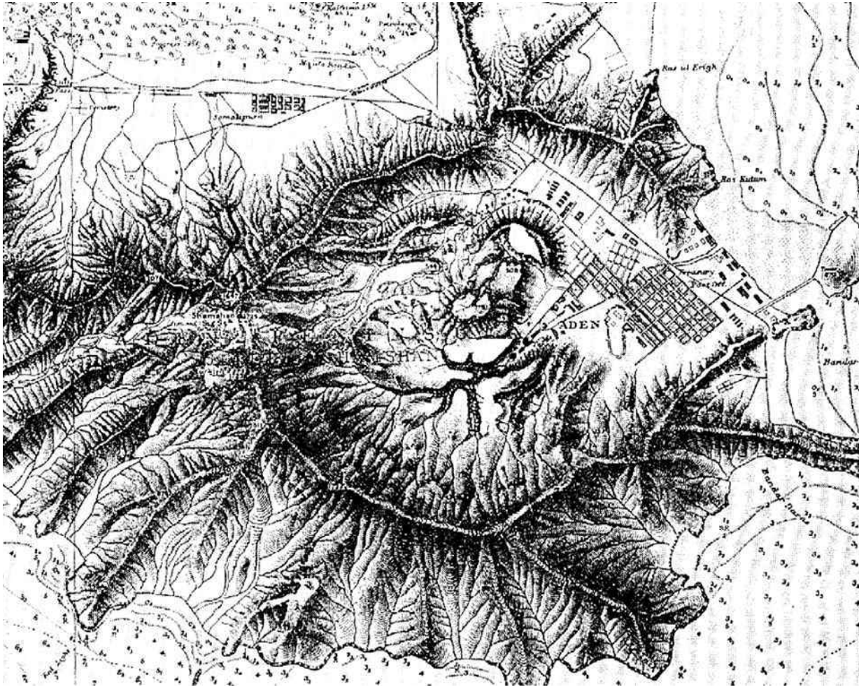
280. Aden (Yemen), situated at the outlet of the crater. Water harvested in the volcanic cone was put in storage in a series of deep cisterns in order to be sold to the ships bound for India. [p. 93]
