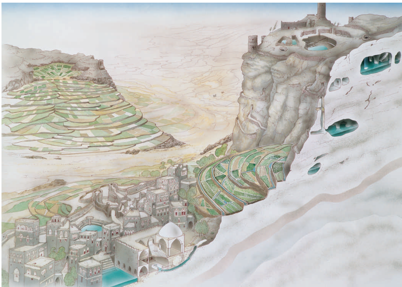
348. Thula (Yemen), reconstruction of water harvesting systems, open-air cisterns, underground cavities and tunnels which from the citadel provide the terraced gardens and the ablution rooms of the mosque with water. The hydraulic installation still in use is very similar to that of the ancient Sabeen towns. [p. 98]
