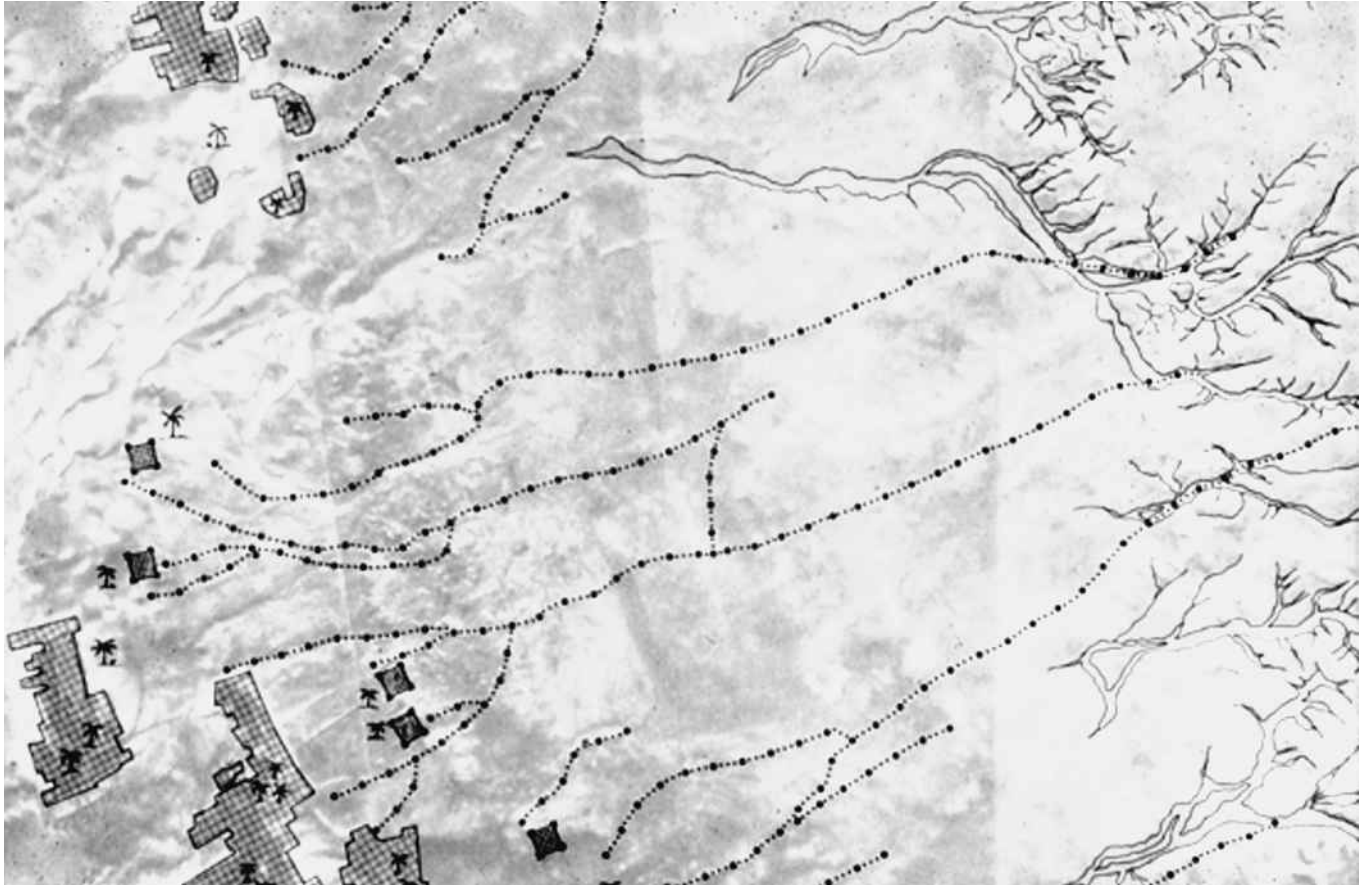
288. Aerial photograph of part of the foggara network supplying the oases of the Sebkhah of Timimoun (Algeria). The underground drainage tunnels, that are evident on the surface from the layout of the excavation shafts, come up from the oases (lower left) and run towards the riverbed of the fossil hydrographical network (upper right). [p. 135]
