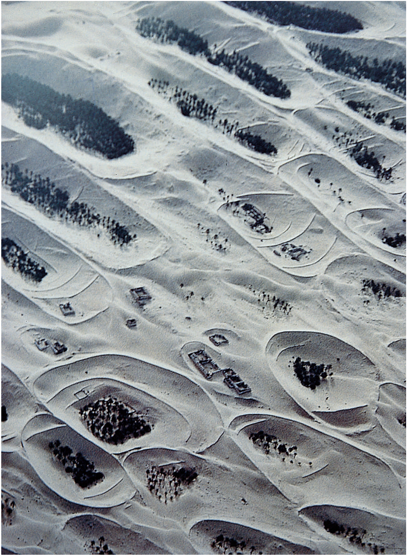
99. The erg oases in the Algerian Souf region with artificial craters (bur) dug out and protected by barriers of leaves, regulate the dune movements and shape the great sandy desert landscape.
