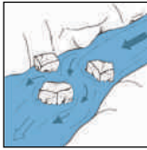
Stones within the streams to reduce the flood strength
