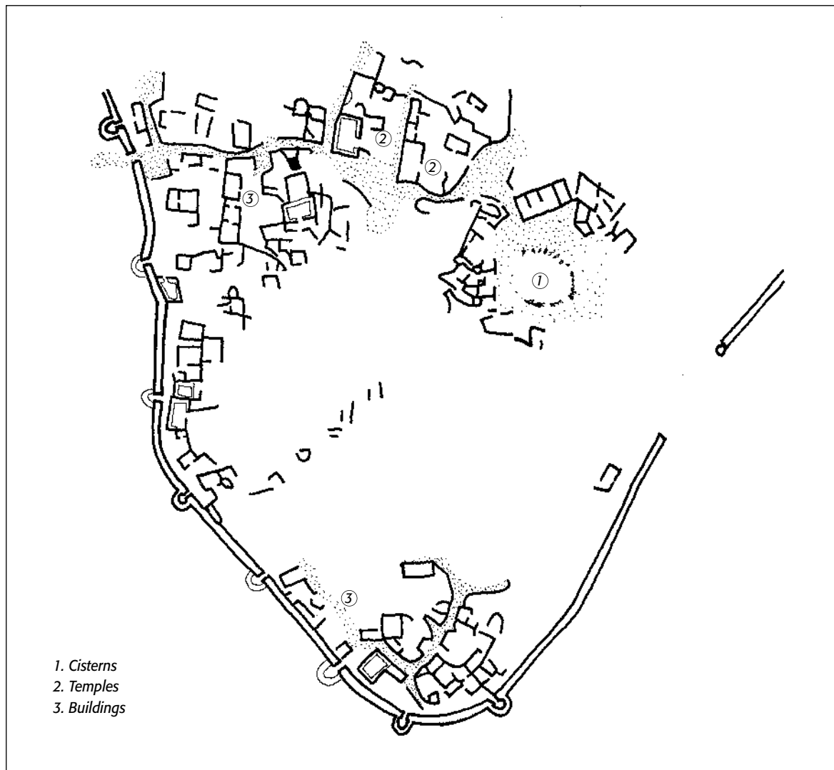
277. Planimetry of the site of Arad in the Negev desert. The early Bronze Age settlement is situated on the hollow top of a hill which acts as an impluvium to collect water for the cisterns surrounded by the built-up area. [p. 89]
