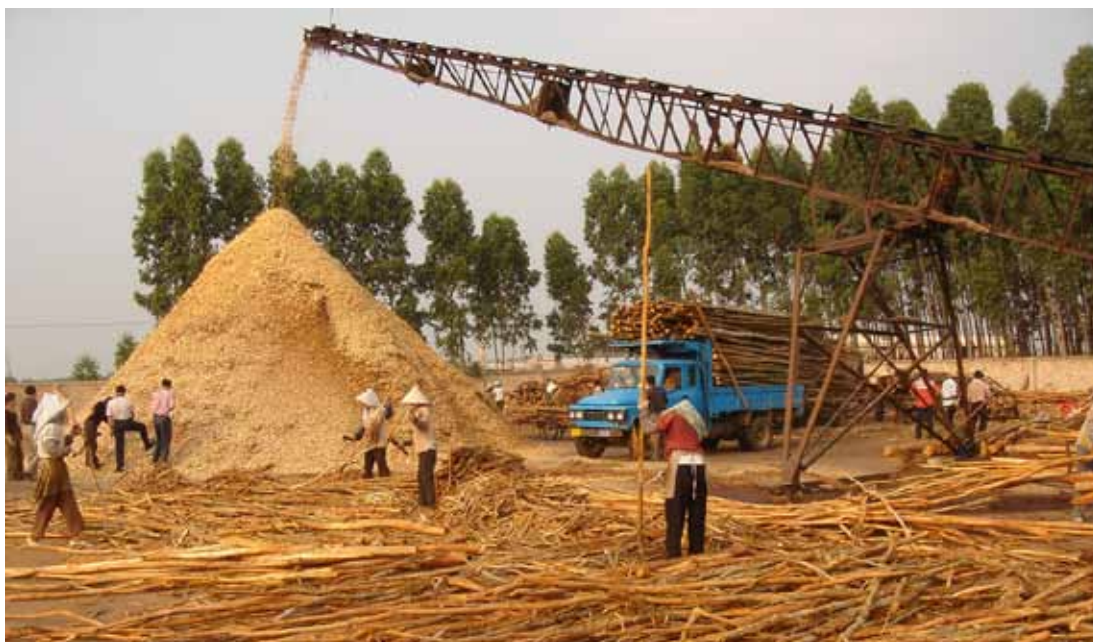
Industrial residues (eucalyptus) processed into chips for use in pulp and paper production. Photo: Jim Carle, FAO (FO-6953).
