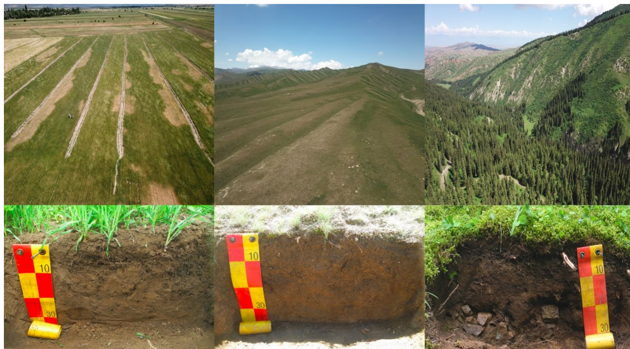
Figure 9: Soil pits in different land-cover classes (from left to right): cropland, grassland, tree-covered area
