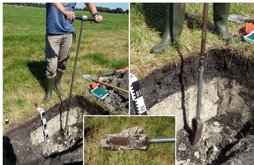
Figure 19: Use of an Edelman drill
