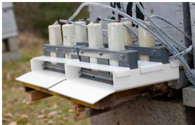
Simulated nicotinoid pesticide exposure of a free-ranging forager honey bee labelled with a radio-frequency identification tag. Credit: © INRA/C. Maitre
